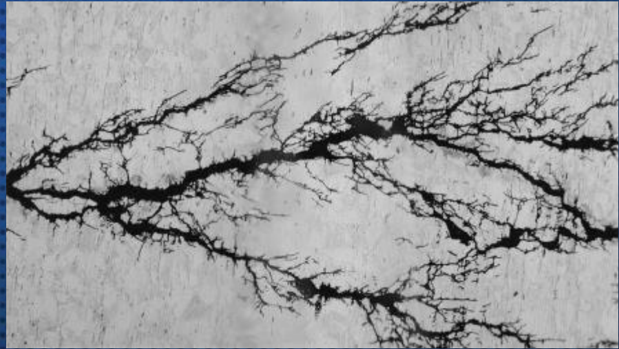
Stress corrosion cracking of stainless steel
