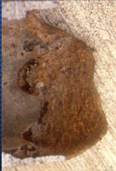
Erosion corrosion for: Check valve (left) and ship rotor blade (right)
