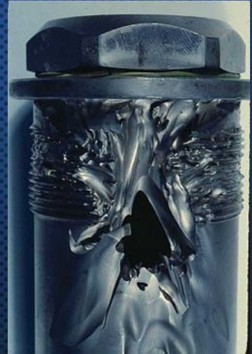
Erosion corrosion for: Check valve (left) and ship rotor blade (right)
