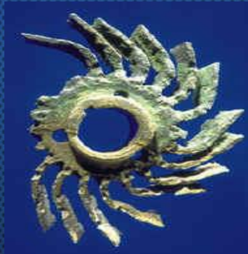
CORRODED ROTOR LEADING TO EQUIPMENT FAILURE
