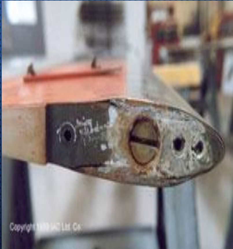
Galvanic corrosion of a helicopter rotor blade
