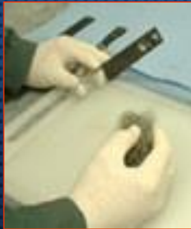
Removal of corrosion product by soft wire mesh
