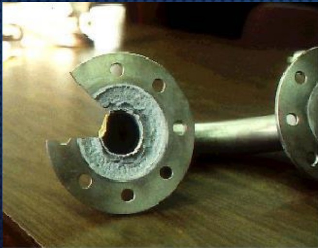
Crevice corrosion of SS
